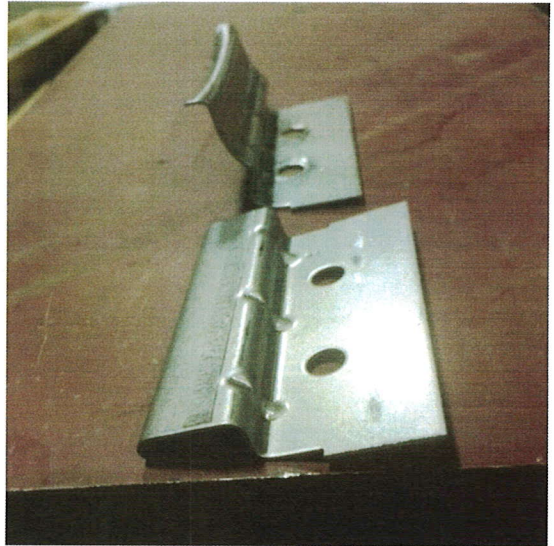
TYPICAL CLIP WITH TYPICAL FAILED CLIP
