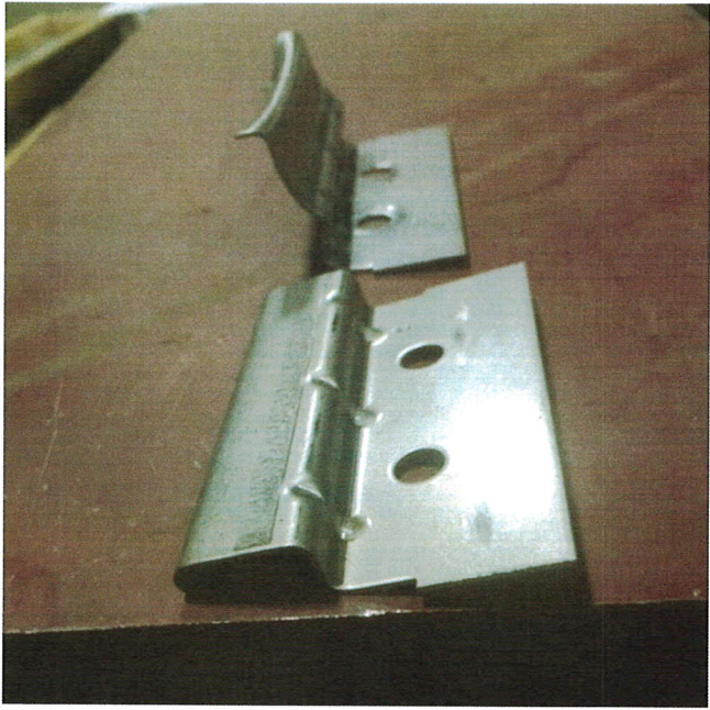
TYPICAL CLIP WITH TYPICAL FAILED CLIP
